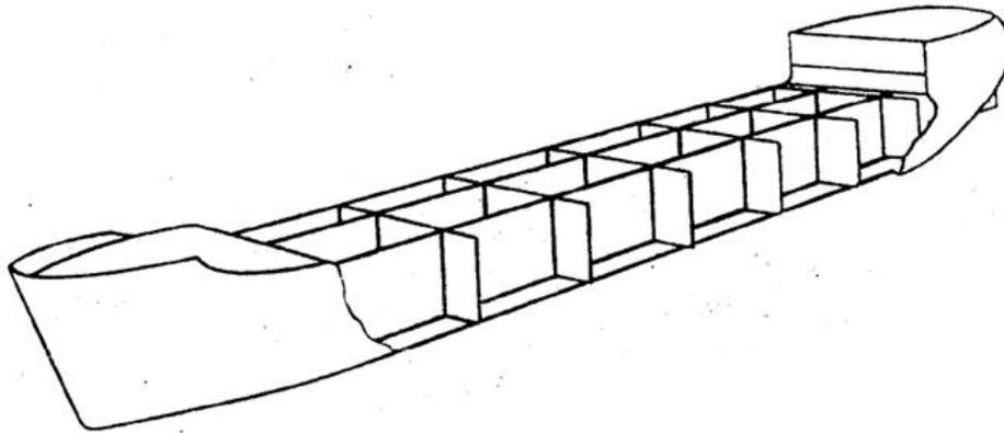
There is a need for an internal watertight subdivision of the hull in compartments to resist the effect of damage (breach) of the hull, or loss of water tightness, and the subsequent flooding is in itself evident.
