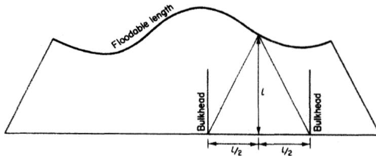
The **ordinate at any point represents the length which can be flooded with the centre at the point concerned**. Thus if 'l' is the floodable length at some point the positions of bulkheads giving the required compartment length are given by setting off distances  $1/2$  'l' either side of the point.
