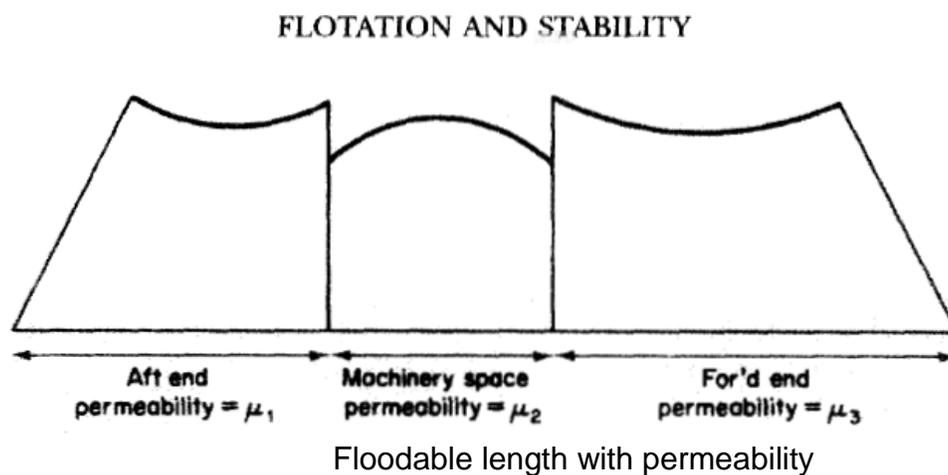
This leads to three curves for the complete ship as shown in Figure. The condition that a ship should be able to float with any one compartment open to the sea is a minimum requirement for ocean going passenger ships. The Merchant Shipping Regulations set out formulae for calculating permeabilities and a factor of subdivision which must be applied to the floodable length curves giving permissible length.
