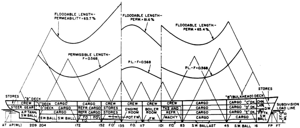
**Fig – Typical F.L and P.L over a ship’s profile**
